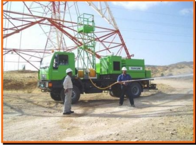
THE CHANCE LIVE LINE INSULATOR WASHER SKID & TRUCK MOUNT SERIES can be fitted to all makes of truck either in factory or in the country of use.
