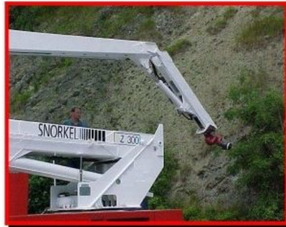
Monitor outputs from 2250 to 6000lpm give throw of foam and water to up to 90m laterally from monitor tip
