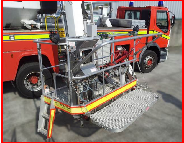
Superb cage access at ground level with fold-down front platform for stretcher & wheelchair rescue with room for 5 adults
