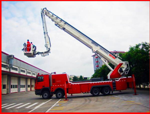
SST-560 on Mercedes Actros chassis with custom fire engineering bodywork and fixed pump installation
