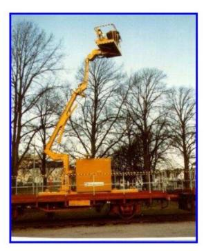
▲The RANGER R-Railway Series is mountable onto a wide range of standard rolling stock wagons, self propelled or rail going vehicles
