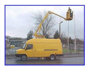
The RANGER R-Light Series is mountable onto a wide range of chassis or van types to suit all applications
