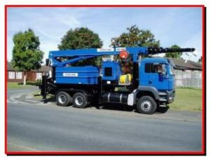
THE CHANCE LIVE LINE INSULATOR WASHER TELE-BOOM SERIES mounts onto a wide range of 3 and 4 axle chassis types to suit all applications. It is available with a skid mounted insulator washer pump and engine module and removable water storage tank up to 10,000 litre capacity with a tele-boom nozzle height to wash to 51m.
