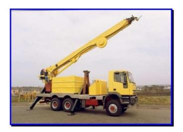
THE CHANCE LIVE LINE INSULATOR WASHER TELE-BOOM SERIES mounts onto a wide range of 3 and 4 axle chassis types to suit all applications. It is available with a skid mounted insulator washer pump and engine module and removable water storage tank up to 10,000 litre capacity with 3 main tele-boom options at 30; 37 and 44m nozzle heights to allow washing up to 51m.
