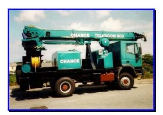
All booms offer proven safe washing on lines up to 500kV with maximum nozzle pressures at 550psi by means of a remote controlled fully articulating nozzle.
